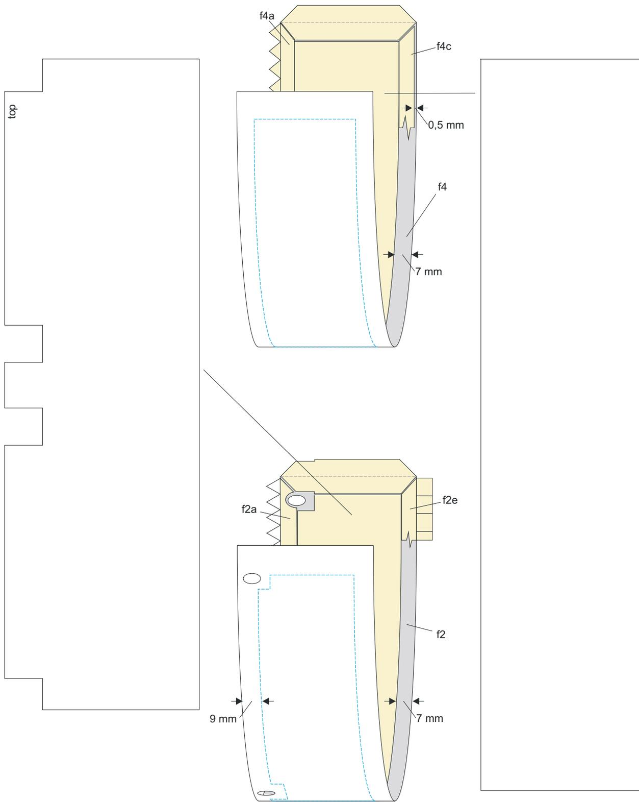
Optional parts for durability of cylinders f2 and f4
